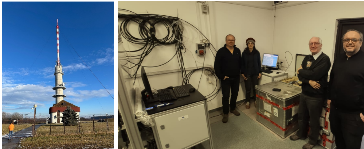
Fig. 3: Sampling at Hegyhátsál tall tower (Hungary, left) by Univ. Frankfurt using a fully automated sampling system (right). The inlet height is at 115 m.
