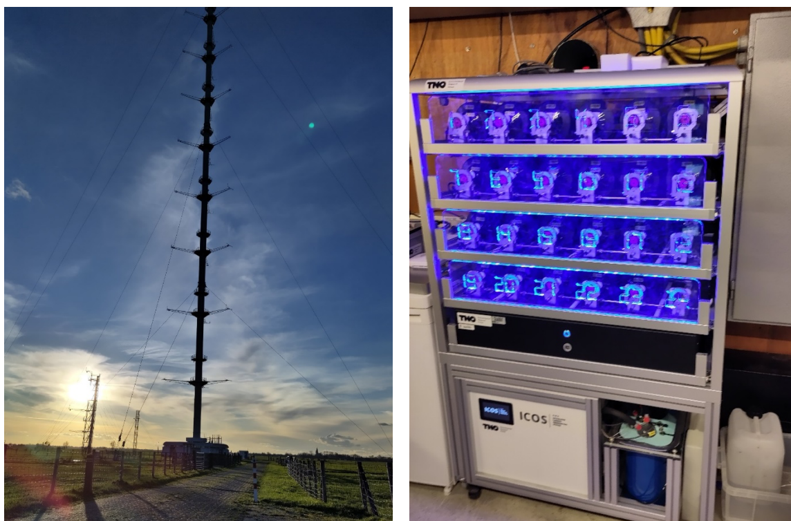
Fig. 2: Sampling at Cabauw tall tower (the Netherlands, left) by Univ. Bristol using the ICOS sampler (right). Air samples are collected from an altitude of 207 m and integrated over one hour.
